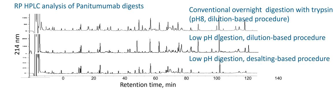
The low pH method can be used in different common sample prep procedures with high efficiency. It can also be readily automated (data not shown).
