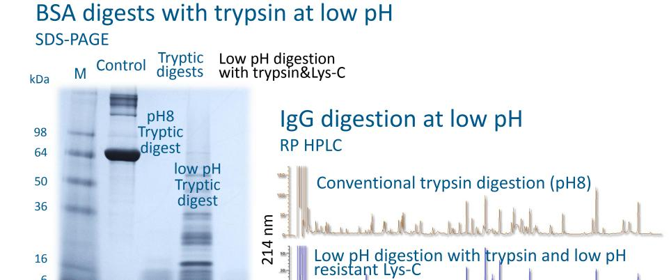
Efficient protein digestion at low pH with trypsin and low pH resistant Lys-C
