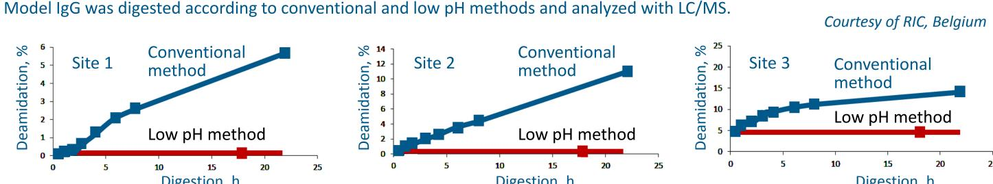
Artificial deamidation is induced over the course of conventional protein digestion reaction. In the low pH method, artificial deamidation is suppressed. Authentic deamidation remains intact.
