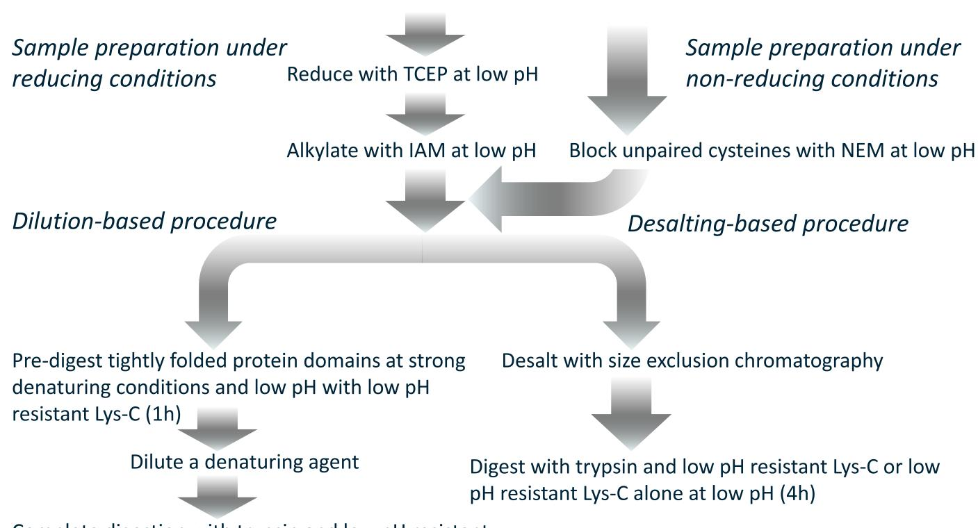
Complete digestion with trypsin and low pH resistant Lys-C or low pH resistant Lys-C alone at low pH (3h)
