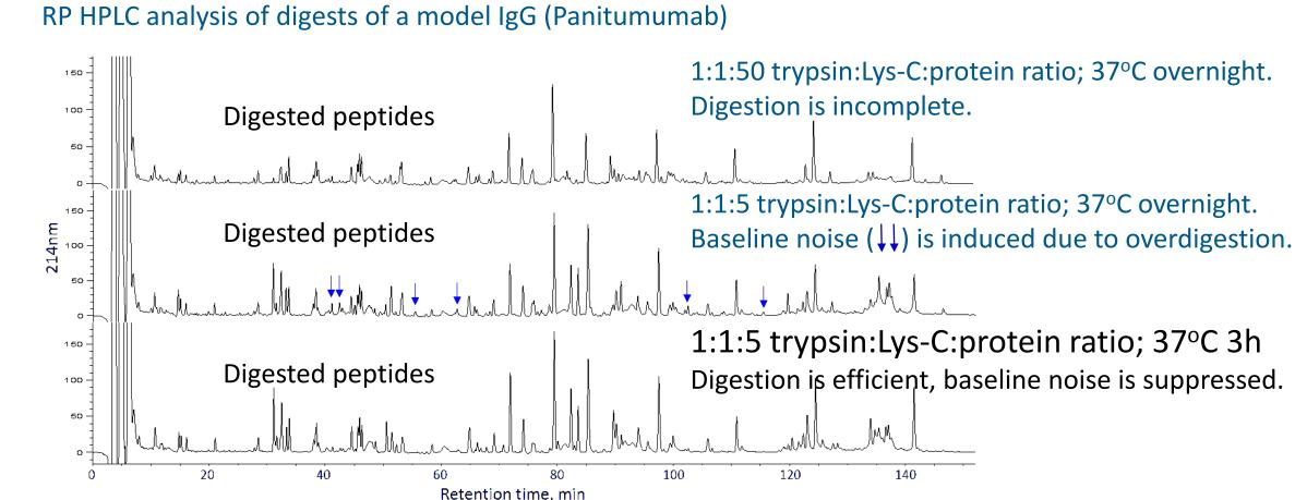
3h digestion at 1:5 protease:protein ratio provides efficient digestion with suppressed baseline noise in the method.
