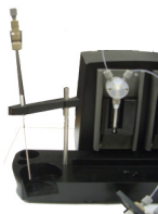
Figure 116. Installation of the inlet tube holder clip.
