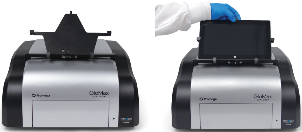
Figure 4. Instrument front and Tablet PC holder setup.
