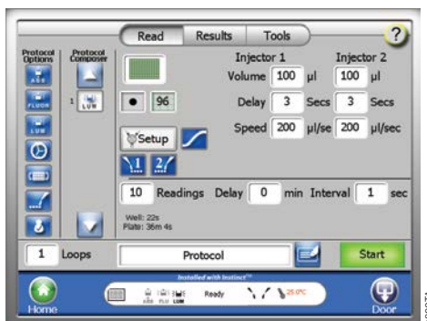
Figure 33. Setting Kinetic Parameters. The “Kinetic” icon is located to the right of the “Setup” button.
