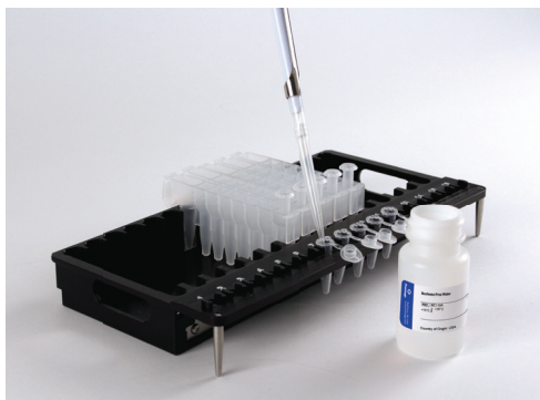
Figure 2. Setup and configuration of the deck tray. Nuclease-Free Water is added to the Elution Tubes as indicated.
