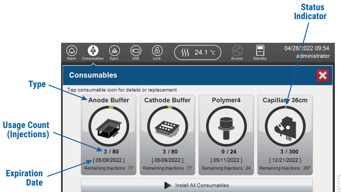
Figure 4. Spectrum Compact CE System 'Consumables' screen. Usage count (number of injections), on-instrument expiration date and remaining injections are displayed on the 'Consumables' screen for each consumable, as well as polymer type.
